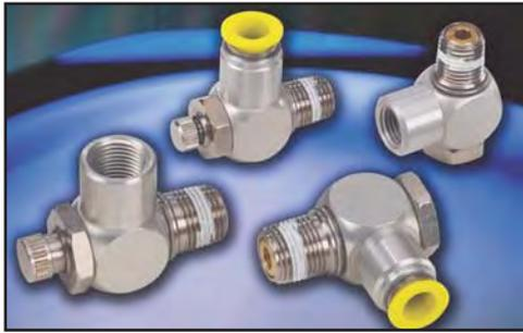
These combination needle and check valve flow controls are typically used to control air flow from air cylinders, thereby controlling the speed at which
